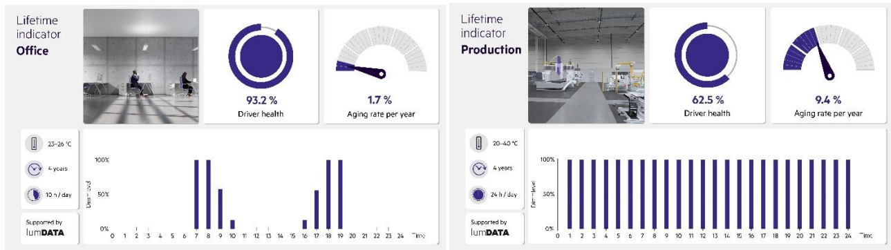
Figure 2: High temperatures, e.g. in production environments, accelerate the aging of LED drivers compared to stable office conditions. (Source: Tridonic)
